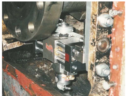
Mounting the "Millgrind" Equipment on a 400 mm \varnothing Main Journal
