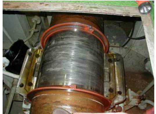
Damaged 505mm Ø Tailshaft Journal
