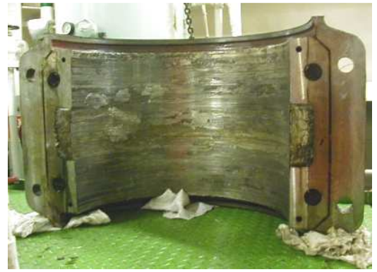
Damaged White Metal Bearing
